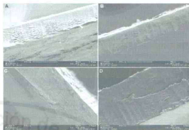
Figure 2. Scanning electron micrographs on cross-sections of free chitosan films containing glycerol (A), erythritol (B), chitosan and Hylon VII (60:40) and glycerol (C), as well as chitosan and Hylon VII (80:20) and erythritol (D).
